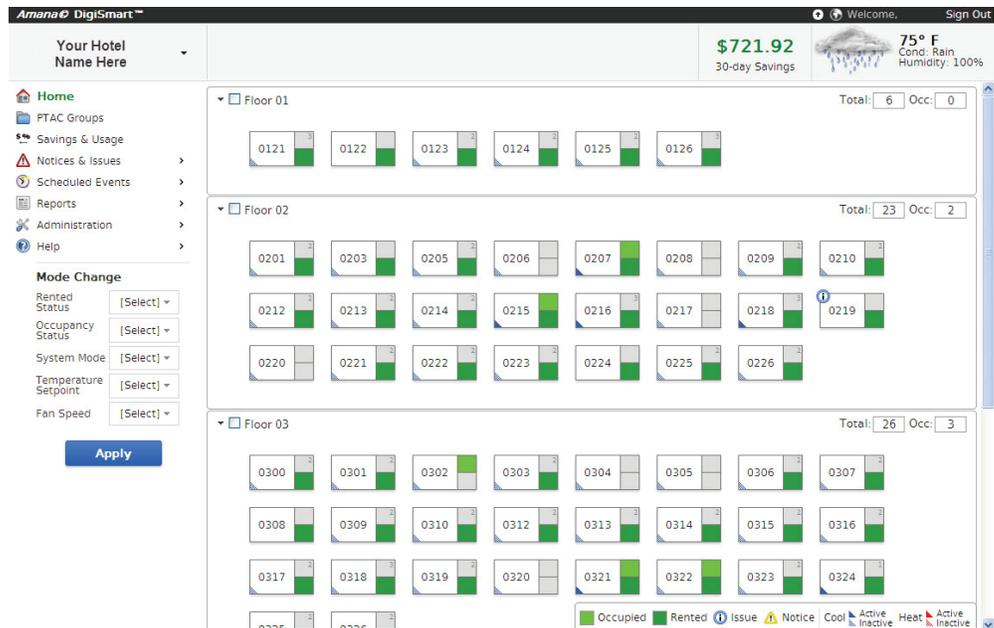
**Temp Limiting** – Each PTAC can be configured with a heating and cooling temperature set-point limit.
